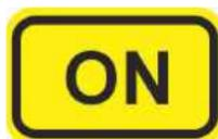
Depressing the ON key will switch the tester "ON". At switch "ON", the tester retrieve the last settings utilized. These are the current/range settings which were last utilized by the Instrument. At Switch ON, the buzzer sounds to confirm the "ON" status.
