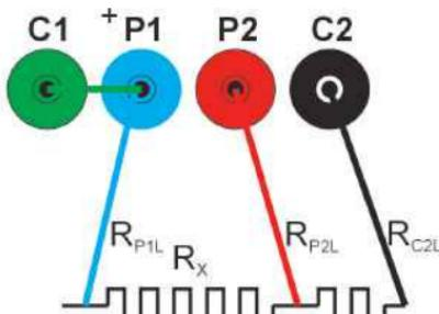
**Using the 3T method,  $R_{C2L}$  does not affect the readings.  $R_{P2L}$  is negligable as no current goes into and P2 but  $R_{P1L}$  is added to  $R_x$ .**
