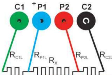
**Using the 4T method,  $R_{C1L}$ ,  $R_{C2L}$  does not affect the readings  $R_{P1L}$  and  $R_{P2L}$  are negligable as no current goes into P1 and P2.**
