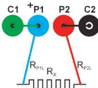
**Using the 2T method, the resistance of the test leads are added to the readings. This is not recommended for low resistance and long leads.**
