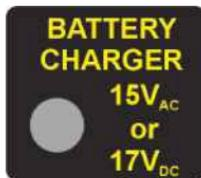
The connector for the Battery charger can accept AC or DC signals up to a maximum of 22Vdc. There is a full bridge rectifier inside the tester, as well as a regulated battery charger. The battery is charged to 13.8V. We recommend the use of the power supply (step down transformer) which is supplied with this tester. The light on the power supply transformer will lights up when the battery charger is working.
