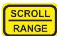
Depressing the SCROLL/RANGE key will stop the test, if in progress, then will change the scale, to the higher ohmic scale (going down on the tester). Depressing the key again will move to the next range etc... Each range illuminate it's corresponding led.
