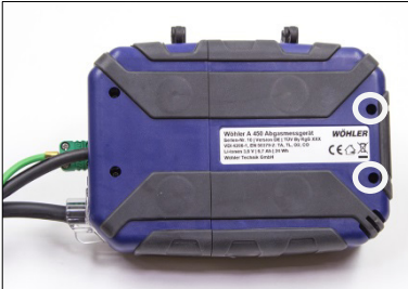
Fig. 50: Bottom of the device - Open the cover by loosening the cross-head screws .
