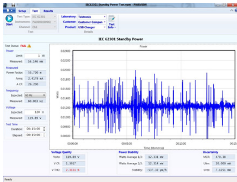
Figure 56: Full compliance IEC 62301 Standby power test
