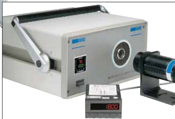
Shown calibrating the OS1552-A pyrometer. Visit omega.com for details.
