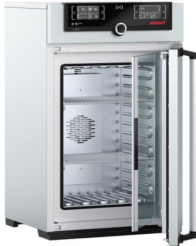
The heating of this incubator is optimally tuned for both natural convection and forced air circulation; the fan can also be switched off completely, and valuable chamber loads for research, pharmaceuticals, medicine and food chemistry are warmed up very carefully.
