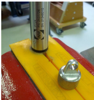
Cableless Sensor—gripping on knurled area
