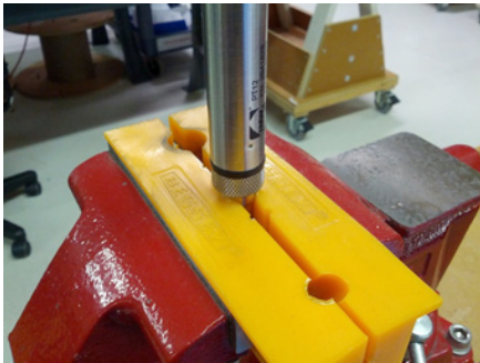
Cabled Sensor—gripping on swage
