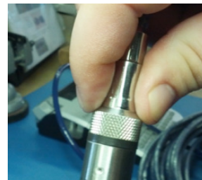
Properly completed—black ring uncompressed
