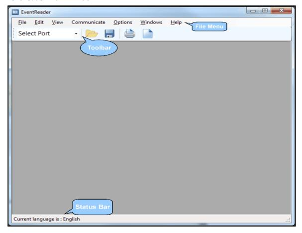
At the top of this window is a menu bar listing various menu selections; below that is a toolbar; and at the bottom of the window is a status bar.
